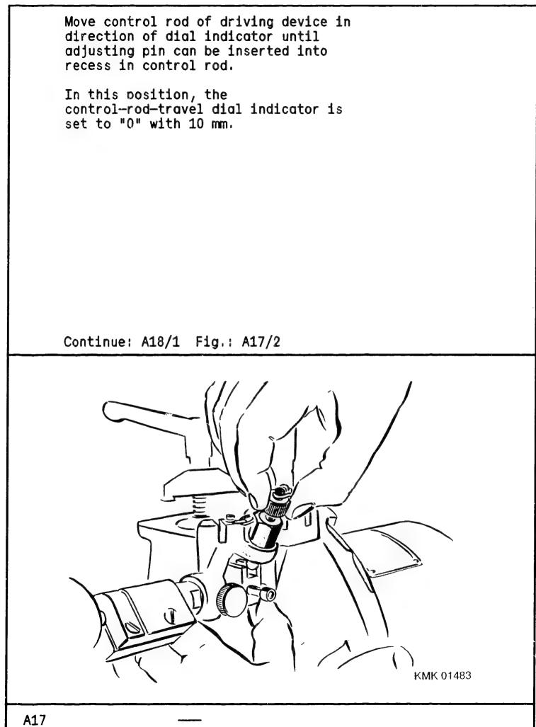
Adjustment of fuel-injection pump Insert fuel-injection pump from top into driving device 1 688 100 078. Use is not to be made of any prestroke shims. When the roller of the roller tappet makes contact with the drive-shaft cam, the fuel-injection pump is still not in contact with the mounting surface. For this reason, continue pressing the fuel-injection pump downwards by hand until it makes contact with the driving device. Place locking claws in position at fuel-injection pump and tighten.
